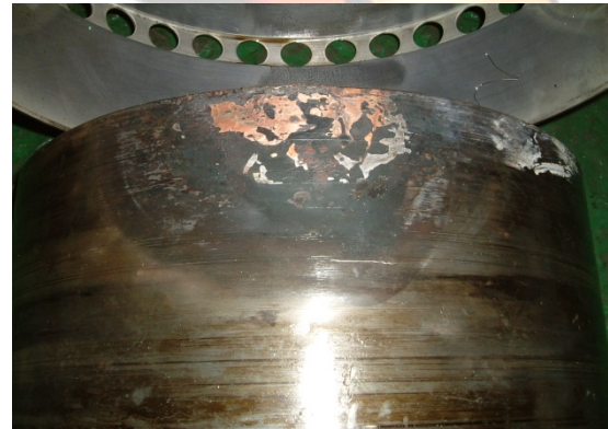
Failed main engine bearings due to poor condition of lubricating oil
