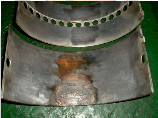
Failed main engine bearings due to poor condition of lubricating oil
