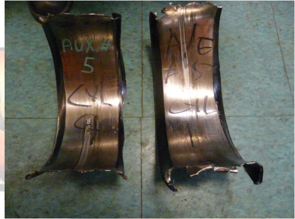
Typical bearing condition – all white metal removed
