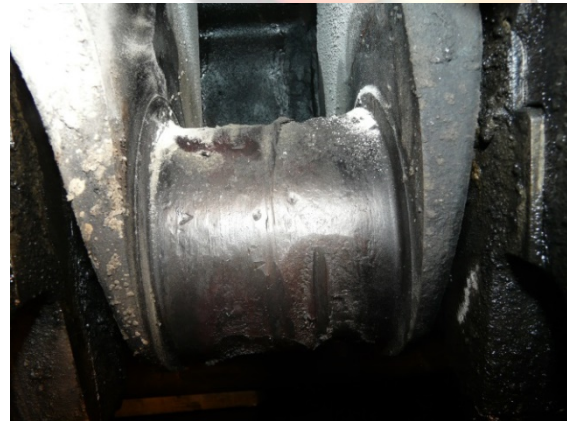
Severe crankshaft damage from breakdown of lubricating oil in a medium speed engine
